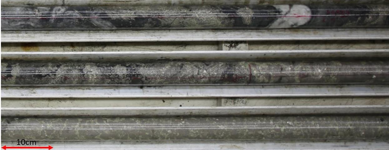
Figure 1: Photo cut-out of core to demonstrate style of sulphide mineralization intercepted in drill hole 16TK0233A (assays pending)
